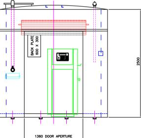
Option D - This will hold a fill point, either 2 x plate mounted pumps or a pedestal pump, alarm and gauge.
